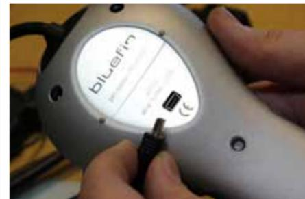
**07** Once this is set up, plug the Bluefin into the computer using the USB lead supplied in the kit
