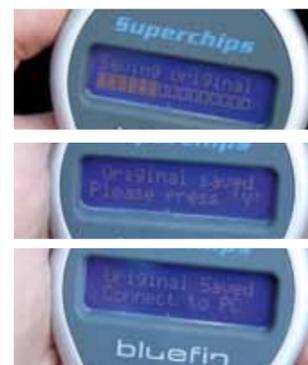
**05** Now, the hand set is reading the original map and saving a copy of it in its memory. Once that is complete, it prompts you to press 'Y' to finalise this part. Having done that, it's time to disconnect from the Van and head inside, to the computer
