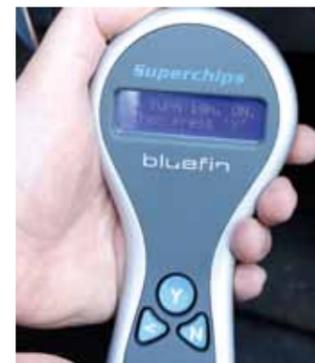
**03** From here on, you basically follow the instructions. Leave the ignition off and press 'Y' on the hand set. At this stage, you're in the 'read' part of the cycle so, if you inadvertently disconnect the Bluefin, you won't have any problems. Once that part of the process is complete, it will prompt you to turn the ignition on and press 'Y' again. However, it also tells you NOT to start the engine
