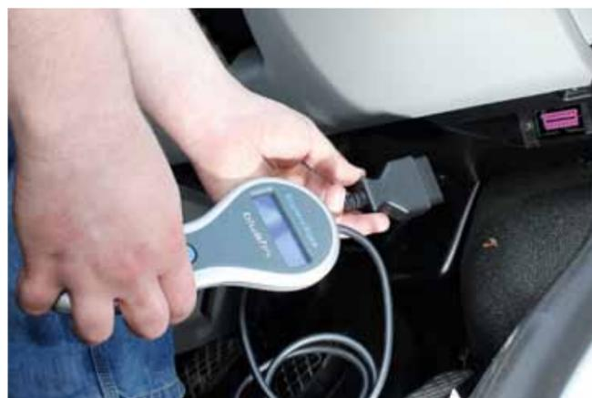
**01** The first thing is to locate the OBD port. By convention, this must be within 1m of the driver and, on the T5, it's under the dashboard, just above the accelerator pedal. Unpack your Bluefin device and connect it to the OBD port. Make sure the ignition is turned off, but keep the key in—you'll need it in a bit
