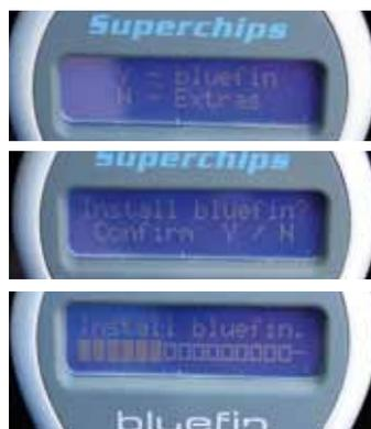
**13** Plug the Bluefin in to the OBD port again and follow the instructions. When prompted, hit 'Y' to install the new map. Hitting 'N' takes you to an extras menu, which includes a very useful fault code reader in case you have any unrelated problems
