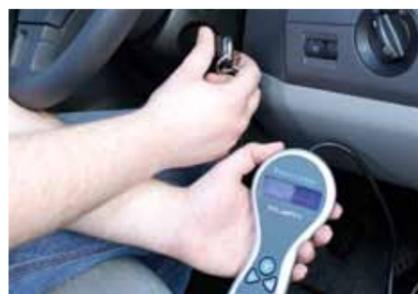
**04** So, turn the key so the ignition is on and hit 'Y' for the next part of the process
