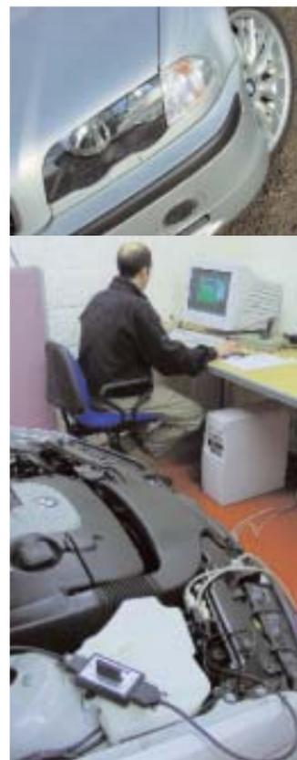
Rewriting the 330d's fuelling parameters requires no component changes and takes half an hour
