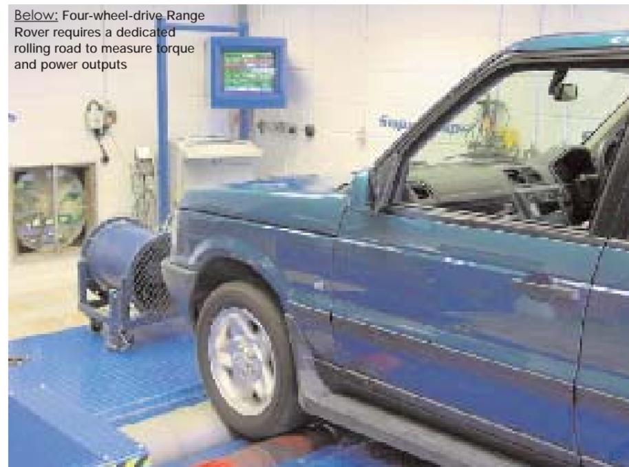
Below: Four-wheel-drive Range Rover requires a dedicated rolling road to measure torque and power outputs
