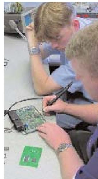
Above: BMW's engine programme chip is replaced by the Superchips item
