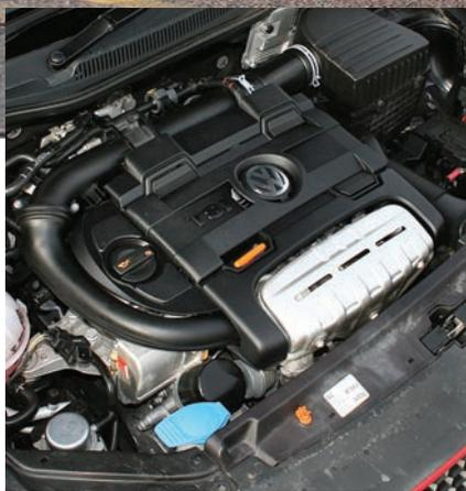
ONE OF THE most interesting engine developments from the Volkswagen Group in recent years has been the twincharged 1.4 TSI unit. Introduced in 2005 and first used in the Mk 5 Golf GT, this small capacity engine uses a combination of direct drive supercharger and exhaust-driven turbocharger, operating sequentially, to boost the power output way above normal expectations for a 1.4-litre engine.
